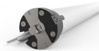
Automate FT15 240V, 15.0Nm, Ø45mm, 15RPM, 621mm long
